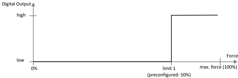
Figure 2: Digital output signal vs. force.
